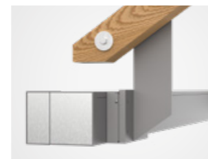
Rafter bracket installation
